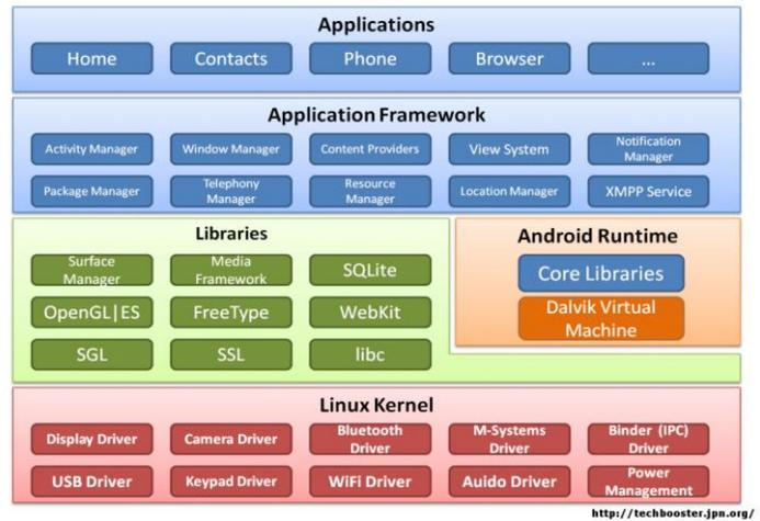
Fig. 4.1 Android Platform Architecture [6]
